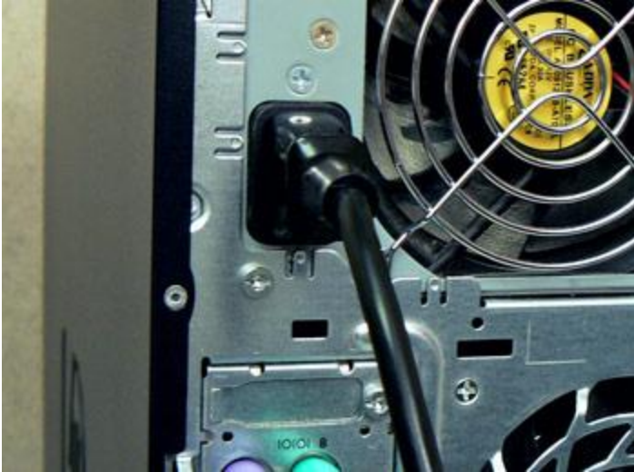
Plug Power Supply Cord into Computer Case
