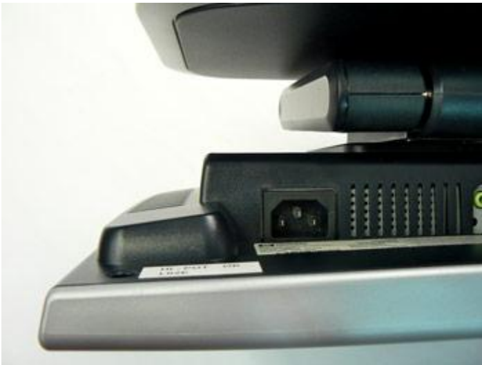
Power Supply Socket on Monitor
